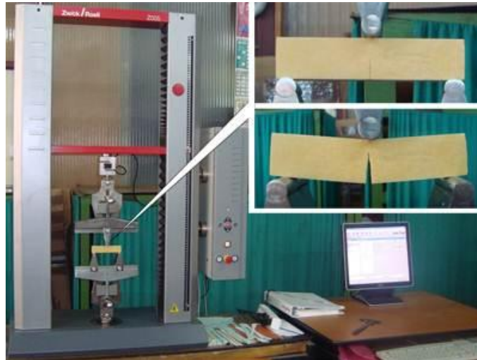
Fig. 27 The 5 kN Zwick Roell 005 testing machine used for 3PB tests
