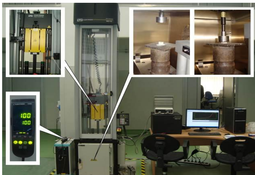
Fig. 14 A Instron – Dynatup 40 kN impact testing machine
