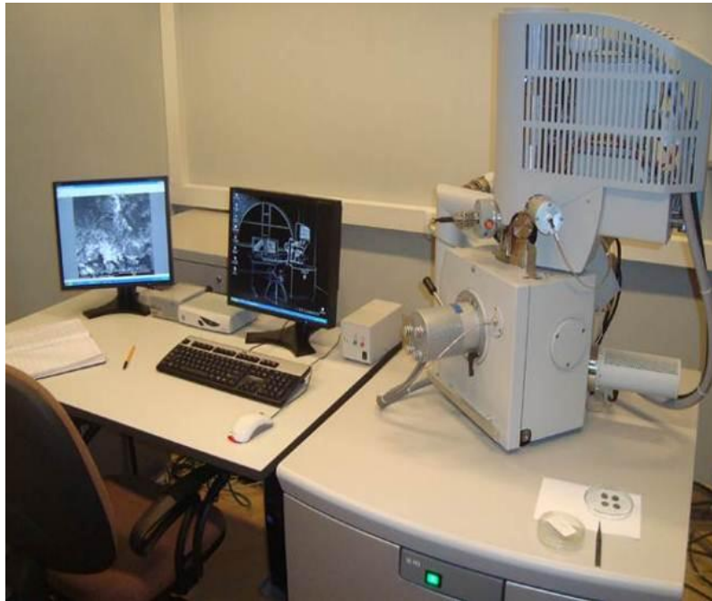
Fig. 45 Scanning Electron Microscope used for microstructural analysis
